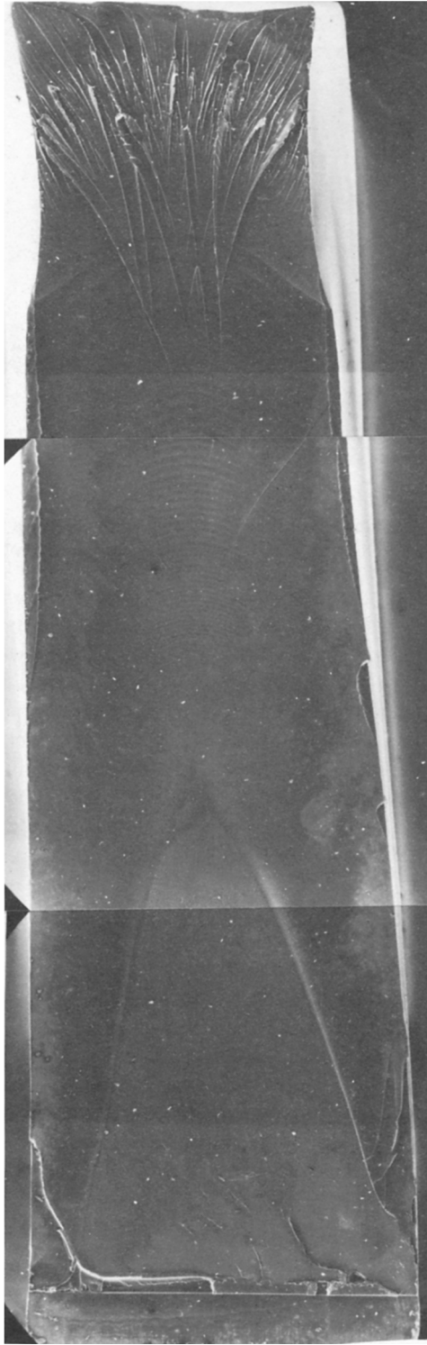
Fig. 9. SEM collage of fracture surface of unannealed specimen cycled at \Delta\sigma = 16.3 \text{ MN/m}^2 . It failed after 5900 cycles.
