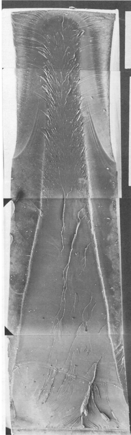
Fig. 11. SEM collage of fracture surface of PC specimen annealed in air and cycled at 12.5 \text{ MN/m}^2 , failing after 22,000 cycles.
